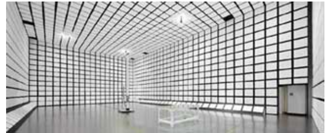
L25m×W14m×H9m Absorber: IP-130BLB(H:1300mm) ANSI: ±3.0dB VCCI: ±1.5dB
